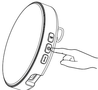
**2. Activate Bluetooth:** Press the Bluetooth button briefly to enable Bluetooth, allowing you to pair with compatible devices. The device Bluetooth name is "E-badge".
