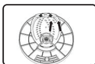
To remove the blade, turn the blade holder over and press the above positions
