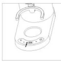
5. When the battery accidentally detaches, the display screen will show an E5 alarm, reminding the battery detachment.
