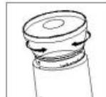
3. The coffee grinder has 60 optional grinding sizes. According to the type of coffee powder required, rotate the coffee bean hopper clockwise and adjust the scale on the coffee bean hopper to the desired grinding size, from coarse to fine.
