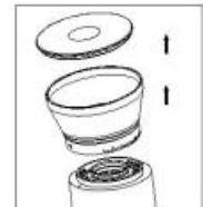
1. Empty the powder hopper, then remove the lid and powder hopper (as shown in the figure).
