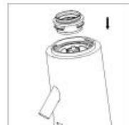
6. Install the coffee bean hopper and its lid in the correct position (as shown in the figure).
