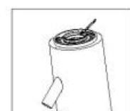
4. Clean the lower grinder with a cleaning brush, or remove any coffee power with a vacuum cleaner.
