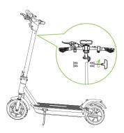
**2.**Firmly connect the wires inside the handle and the stem.
