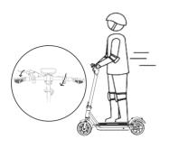
Slow down by releasing the throttle and brake by squeezing the brake lever.
