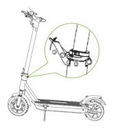
**3.**Install six screws (two on each side) with the included hex wrench.
