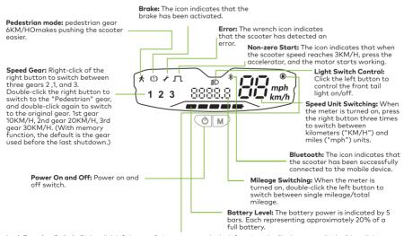
**Lock Function Switch:** Right-click left button 8 times to open the lock function, the "lock scooter display" icon lights up, and the motor can't turn in the locked state. Press the left button again 8 times to unlock the scooter.
