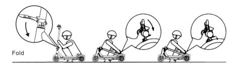
Make sure that the power of the electric scooter is turned off, open the folding mechanism, put down the pipe, and hook the handlebars onto the rear fender. When opening, press the hook at the rear fender until the handlebars can be released, then unfold the electric scooter.
