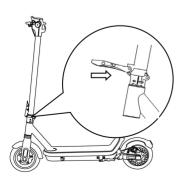
Install the throttle brake with the handlebars (R and L).
