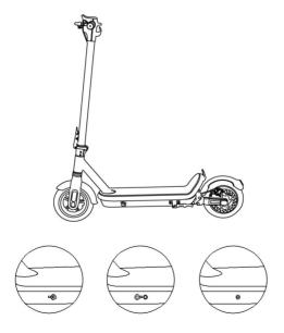
Open the rubber Insert the charger After charging, cap on the port. into the port. put the cap back.
