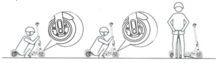
If the tire has gone down, remove the cap on the inlet, connect it to an air pump to inflate it.
