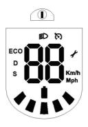
**2.** Current Gear: Double press the switch to change gears between the first (ECO), second (D), and third (S) gear.
