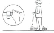
Do not press the accelerator when you are walking on foot.
