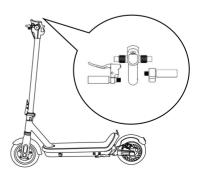
Install the handlebars with the pipe (R and L). Lock the throttle brake screws.
