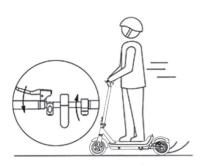
4. Release the accelerator to slow down. The energy recovery system will be automatically activated. Squeeze the brake lever at the left handlebar to stop the scooter.
