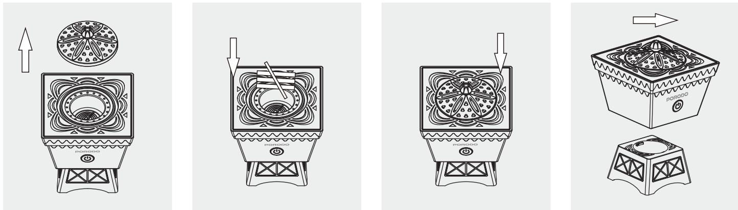
**4.** The bottom part is the incense storage chamber. Rotate clockwise to open, so you can place charcoal or wood. Rotate counterclockwise to close.
