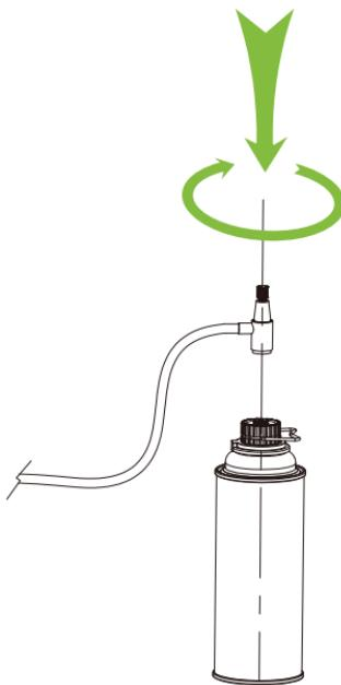
5. Press down on the adapter and rotate it clockwise by 5-10°.
