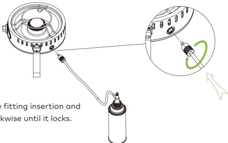
7. Align the fitting insertion and rotate clockwise until it locks.
