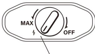
Clockwise rotation is the direction of closing the valve
