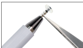
Solution 2: By Scissor/Tweezers- Clamp the Metal tube with Scissor/Tweezers and pull the tip out lightly (Do not clamp the rubber Joint)
