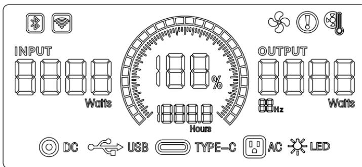
The LCD screen will display both the charging and discharging status of the product. While in use, it will show the remaining battery power.
