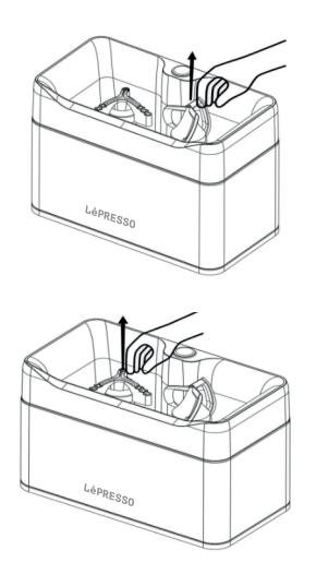
3. Lift the body upwards in the direction of the arrow to complete the disassembly.
