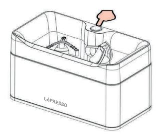
2. As shown in the figure, gently lift the brush head using your fingers to easily remove it, following the direction of the arrow.
