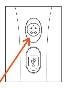
The indicator light inside the switch button will flash while charging and remain steady once fully charged.
