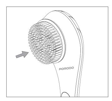
Step 2: Press firmly to complete the assembly.
