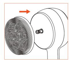
Step 1: Place the replacement brush head according to the direction of the arrow.
