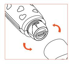
Step 1: Rotate the battery cover and pull to remove it.
