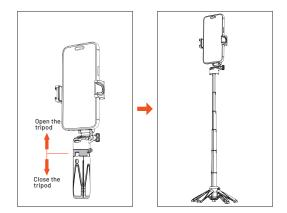
To open or close the tripod, pinch and push the electroplated part of the tripod either downward or upward depending on your desired action.
