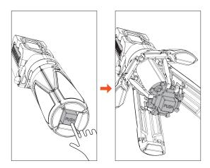
Find the "PUSH" button at the bottom of the handle and press it. The four legs will automatically extend forming the tripod base.
