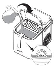
1. Remove the basket and add water up to the "MAX" water level.
