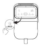
6. Press the "ECO" mode to select the setting where the ice maker will stop for 40 minutes after the ice basket is full.
