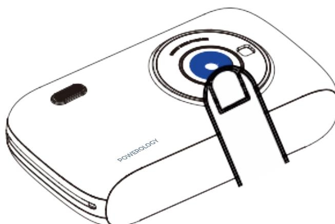
**2. Insert the consumable into the compartment, following the orientation indicated below. Place your finger in the "Push" position and press until you hear a "click" sound.**
