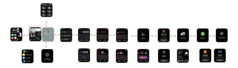
**3.** After turning on the smartwatch, the watch face will appear. Press and hold for 5 seconds to select a different clock face of your choice.
