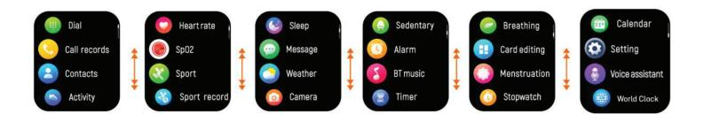
1. Dial: Tap this function to enter the dial interface. Pair your mobile phone with the watch by enabling Bluetooth on your phone and searching for the device name of the watch. Once the pairing is successful, you can make calls directly from the watch.
