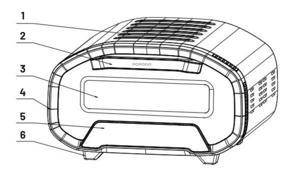
1. Housing 2. Handle 3. Glass Door 4. Frame 5. Control Panel 6. Base
