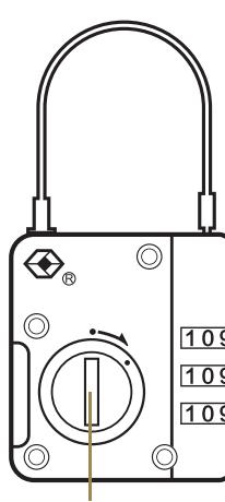
Open this cover to access and replace the battery when needed.
