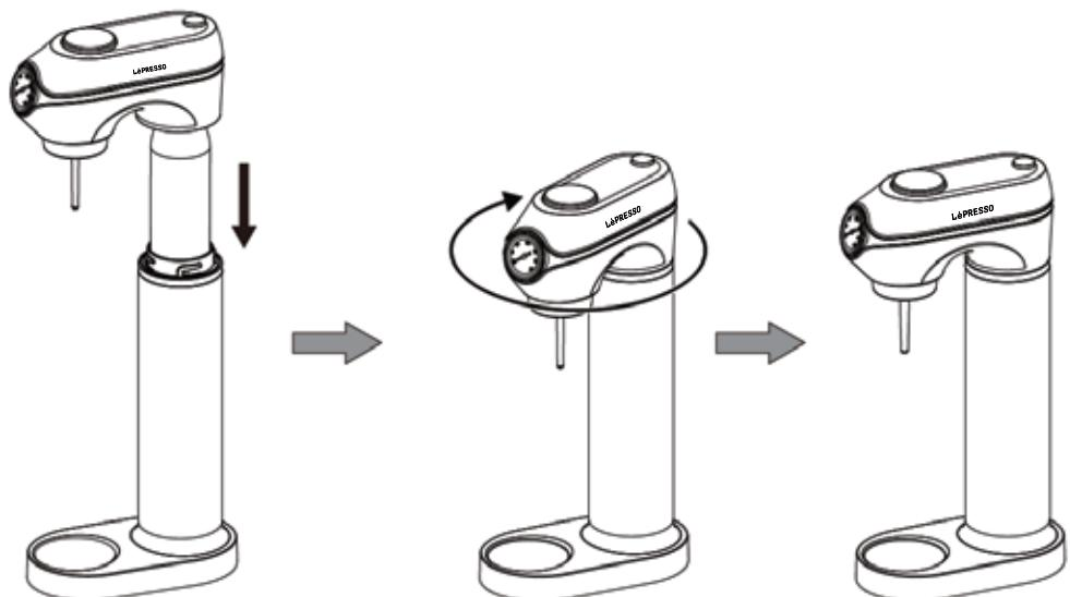
**5. Before first use, rinse the bottle thoroughly. Fill the PET bottle to the designated fill line, indicated between the Min and Max markers. Securely attach the PET bottle to the bottle holder located on the upper housing.**
