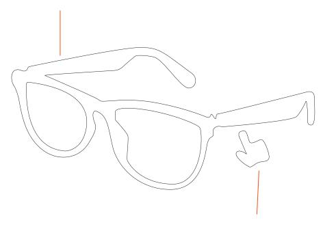
**Power On:** Press and hold the multifunction buttons on both temples for 3 seconds to turn on the device.
