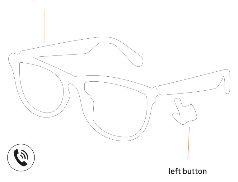
Answer or End a Call: Short press the left or right multifunction button once. Reject an Incoming Call: Press and hold the left or right multifunction button for 2 seconds.
