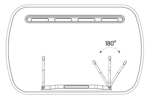
The spring book clip can rotate up to  $360^{\circ}$ ; however, it is recommended not to exceed a  $180^{\circ}$  rotation during use.
