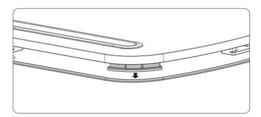
Completely remove the steel ring from the slot.
