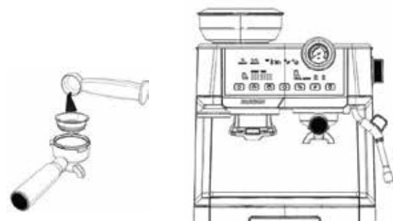
5. Pressing the "Double Cup" button causes the machine to brew two cups of coffee, stopping automatically when finished.
