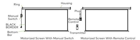
If the motorized Screen Work with remote control, please refer to the diagram below foe electrical connection.
