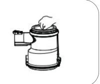
**Step 3:** Remove the filter case, then take out the filter.
