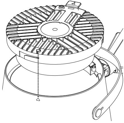
**2.** Once the fan is positioned within the casing, rotate it following the direction indicated by the icon until it clicks into place, confirming it is securely locked. To disassemble the fan, rotate it in the direction opposite to the icon to unlock and remove it.
