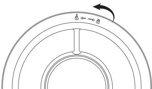
**1.** Find the triangle sign on the product case and the lock icon on the air inlet mask. Align these markers precisely to ensure they fit perfectly into the housing after vertical alignment.
