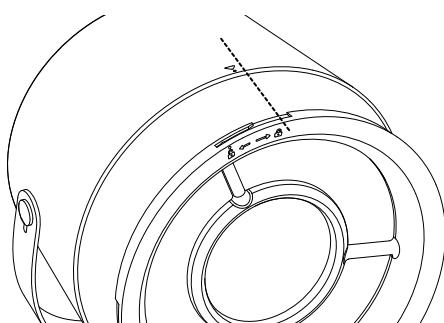
**2.** After positioning the mask within the case, follow the direction indicated by the icon and rotate it until it clicks securely into place. To remove the mask, rotate it towards the icon's direction to unlock and gently pull it out.
