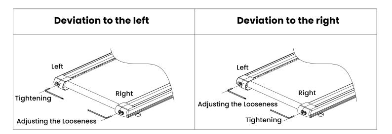
Warning: Running the belt off track can seriously damage the belt and affect its service life. Please make timely adjustments if deviation is found.
