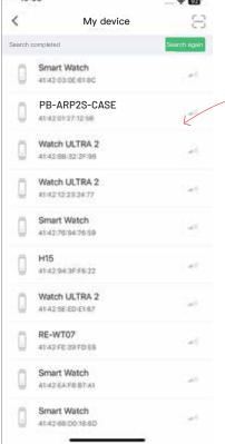
Click to connect the charging case. After connecting, open the top cover but do not immediately remove the headphones. Wait for three seconds to allow the headphones to connect automatically.
