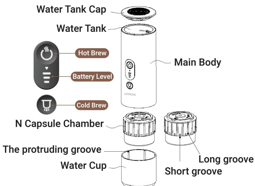
The protruding groove of the water cup connects with the short groove, creating space between the main body and the water cup to collect the extracted coffee.
