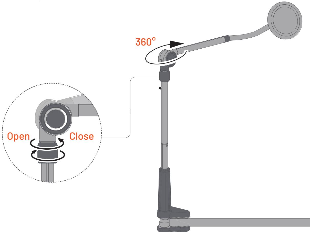
**5.** When making vertical adjustments, slightly lift the arm first, then press the circular button to adjust vertically. There are approximately 15 gears in total, each with approximately  $12^\circ$  adjustment range, allowing for a total vertical adjustment of  $180^\circ$ .
