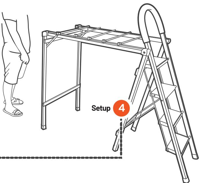
**2. Securely tighten the triangle link to make sure there are no loose parts.**
