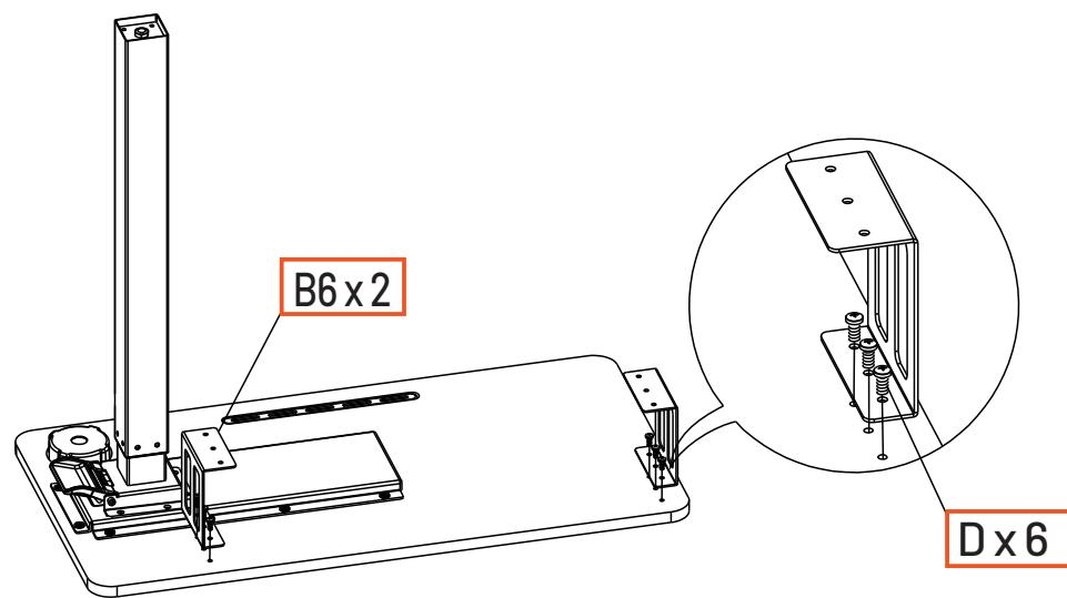
**! Note:** The two keyboard connection panels should face inwards and its smaller side should be fixed to the rear end of the desk, as shown in the picture.
