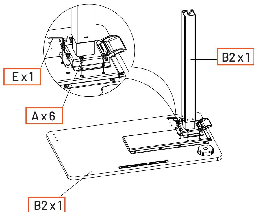
**! Note:** The handle of the desk should face upwards, as shown in the picture.
