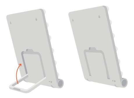
**Step 3:** The mirror can also be mounted on the wall by utilizing the two wall mount holes located on the back.
