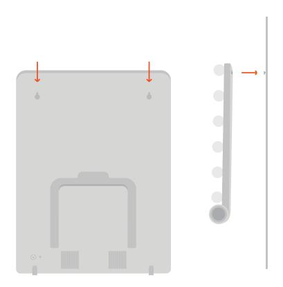
**Step 4:** Make sure there is enough space behind the mirror to easily plug it in using the provided power cord, ensuring access to a reliable power source.
