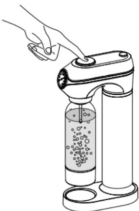
7. Press the exhaust button to release excess CO<sub>2</sub> until the pressure gauge shows 0.
